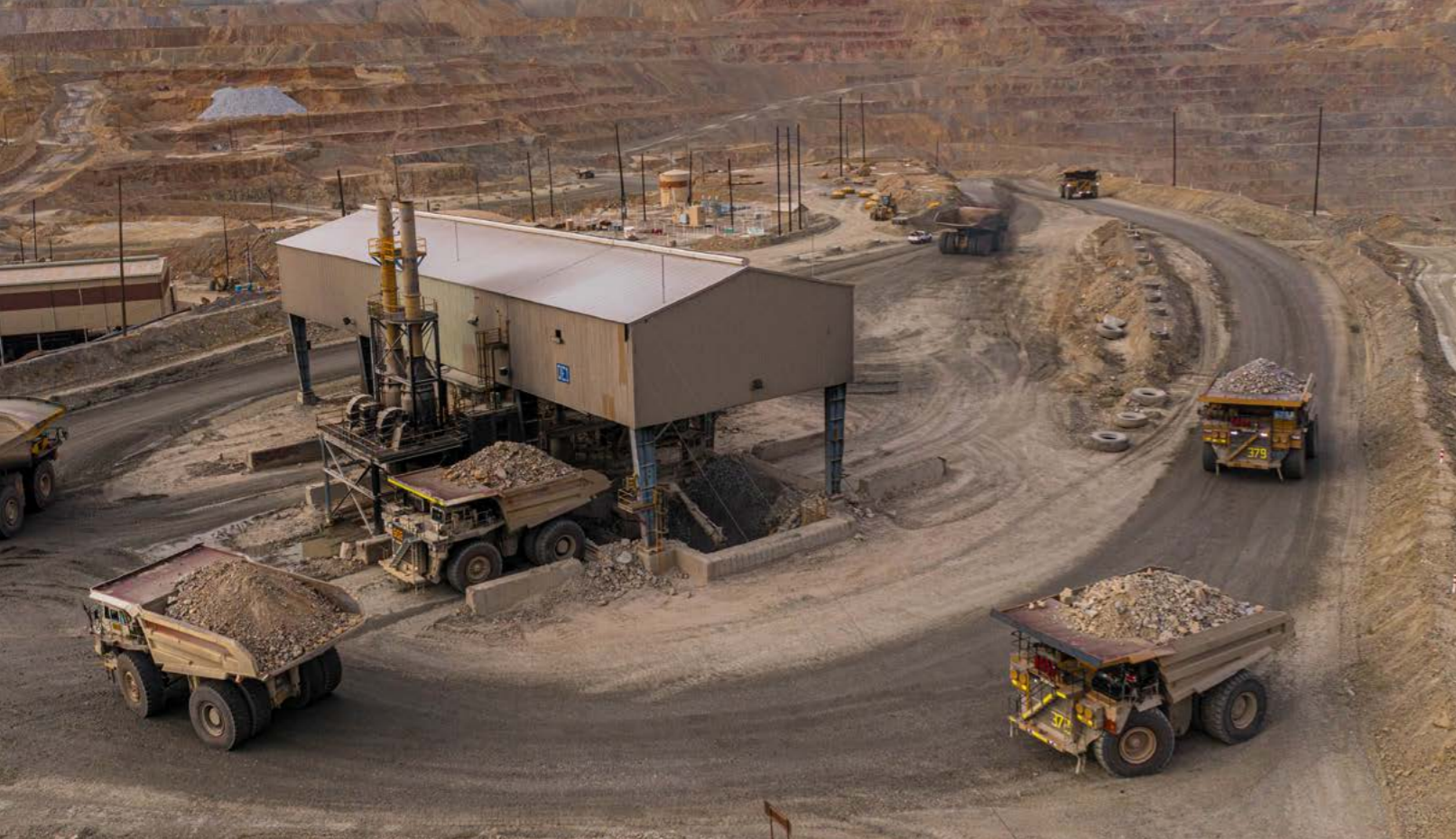
Energy-saving mining trucks with up to 440 tons capacity at La Caridad mine in Nacozari de Garcia, Sonora, Mexico.
